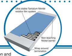
The IRC TaNFilm® PFC chip resistor series provides the high precision and ultra stable performance of our Tantalum Nitride resistive film system in 0603, 0805, 1206, 1505, 2010 and 2512 sizes. The unique characteristics of the passivated Tantalum Nitride film insure long term life stability and stability in moist environments.
